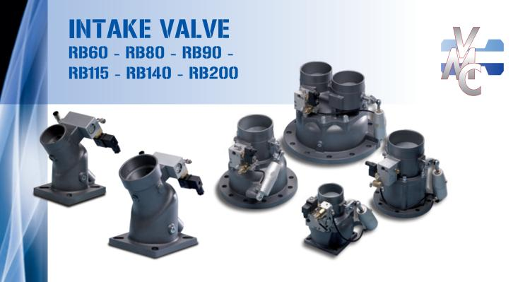
**APPLICATION:** Installed at the compressor inlet to control compressor capacity. During normal operation the valve open and close in response to a control signal to meet the air demand. Stepless or two point capacity controls are available. At the shut-down a check valve stays closed to prevent back flow through the compressor also if the air flow is interrupted. Many solutions are available for stationary or mobile compressors.
